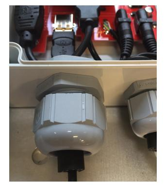
Step 11 - Firmly screw the large nut back on to the plug. Ensure that you do not over tighten this to the point of causing damage to the plug or nut.
