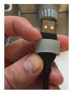
Step 6 - Insert the USB cable of your Oculus through the grey rubber insert from the large plug.
