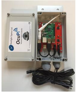
Step 1 - Using a suitable screwdriver, push down and turn the 4 screws on the lid of the Ocupi anti-clockwise approx. 90 degrees until they pop up and release.
