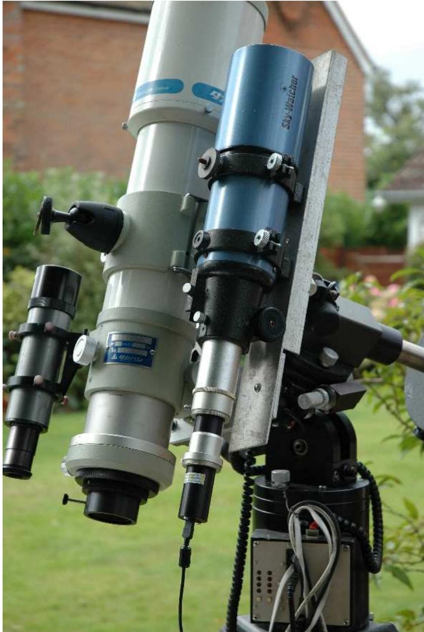
The CoStar attached to an 80mm F5 guide 'scope
